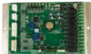
Unit Control Board Within the AAON Rooftop Unit
